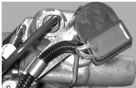
Position Sensor view from rear of Transmission
